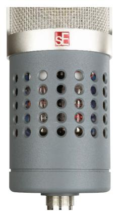
Like its predecessor, the Gemini II boasts twin valves, one for the input stage and one for the output stage, which can clearly be seen through the mic's case.
