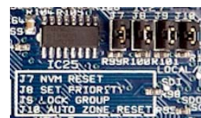
J6 Jumper – Internal Speaker (on/off) J7 Jumper – None-Volatile Memory (resetting) J8 Jumper – Making Mic Priority (DCM1 Only) J9 Jumper – Group Lock (on/off) J10 Jumper – Auto Zone Reset (on/off)
