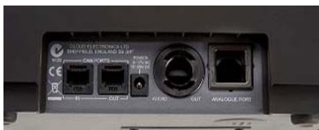
RJ45 Connectors – DCM1 or Analogue Connectors Z8 (or any 3 rd Party System)
