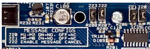
J20 Jumper – Message Triggers 1-2 (NO/NC) J21 Jumper – Message Triggers 3-4 (NO/NC) J22 Jumper - Message Triggers 5-8 (NO/NC)
