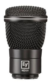
The microphone head features an innovative capsule shock-mount system consisting of a 4-point suspension around the circumference of the capsule combined with a tuned pneumatic pump at the capsule base, offering superior handling noise reduction to eliminate mechanical vibrations and noise in the mix.
