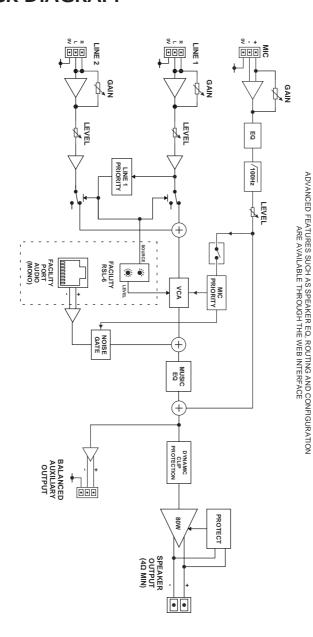
BLOCK DIAGRAM SHOWN IN "OUT OF THE BOX" MODE
