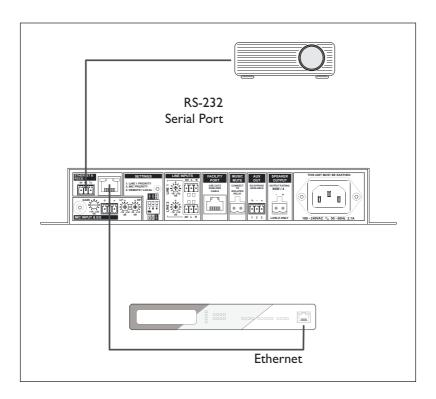
This function uses the MA80E's virtual CDI port, whose address has the default value of 4998. If the controlling device is only able to support remote ports in a certain address range (i.e., not including 4998), the port address can be changed on the **Network Configuration** page of the browser interface (select **Config** > **Network**).
