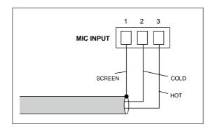
The MA80E's microphone pre-amplifier is an electronically balanced, transformer-less design configured for optimum low noise performance. The input impedance is greater than 2 kohms and is suitable for microphones in the 200 ohm to 600 ohm range. The microphone signal path includes a fixed high-pass filter. This attenuates the response below 100 Hz, which helps to reduce the effects of microphone handling noise.
