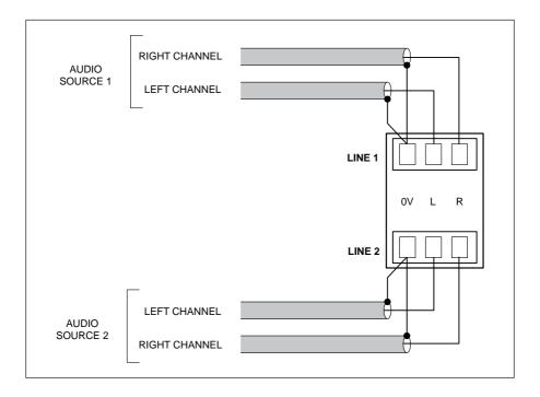
Unless a Cloud remote control plate or module such as the RSL-6 or LM-2 is in use, the two line inputs are summed together internally, though Line input 1 can be configured to have priority over Line input 2, see "Line 1 Priority" on page 22
